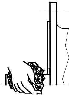
1. Cleaning the motor shaft
