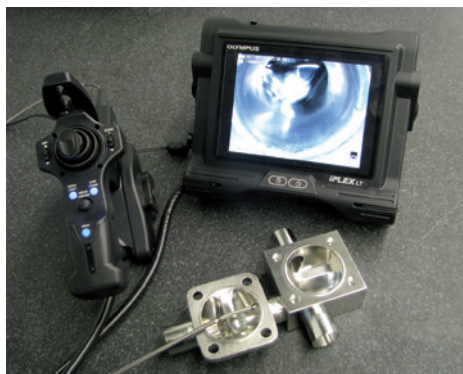
Borescope inspection of the interior surface and weld seams of valves for aseptic applications
