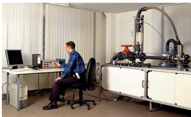
Test stand to determine and document flowrates and K_V ( C_V ) values
