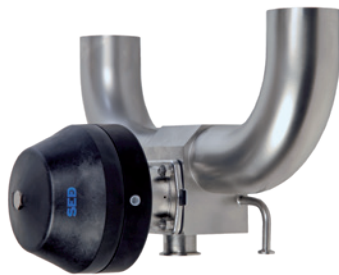
MZ - Multiport Valve T-valve with U-bend and sample valve Main valve KMA Series pneumatically operated Sample valve Steripur Series manual
