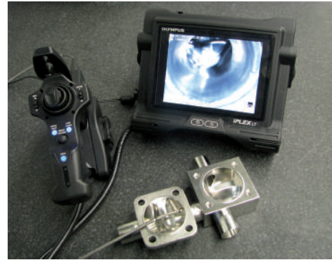
Borescope inspection of the interior surface and weld seams of valves for aseptic applications
