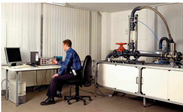
Test bench to determine and document flowrates and K_V ( C_V ) values
