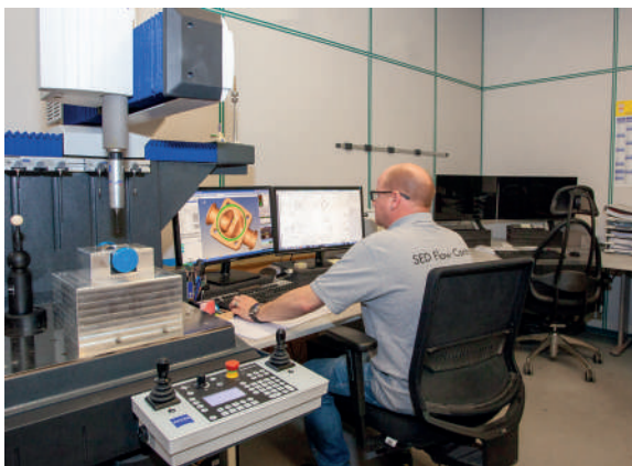
Zeiss Coordinate measuring machine (CMM)
