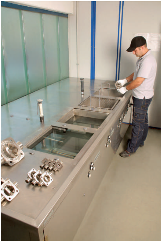
Ultrasonic cleaning of valve bodies
