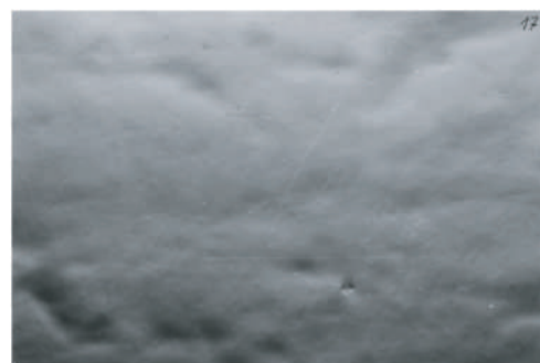
Microscopic view of mechanically polished and electro polished Ra 0,25 µm / 10 µ-inch
